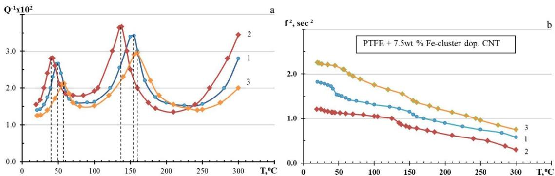
**Fig. 1.** The amplitude-independent internal friction  $Q^{-1}(T)$  – (a) and shear modulus.  $G \sim f^2(T)$  – (b) temperature spectra of the nanocomposite PTFE+7.5wt% Fe-cluster-doped CNTs sample, measured before (curve 1) and after (curve 2) cycling deformation and post-deformation annealing as well (curve 3).
