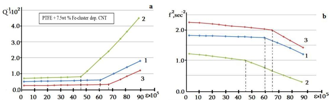
**Fig. 2.** The amplitude-dependent internal friction  $Q^{-1}(\epsilon)$  – (a) and shear modulus  $G \sim f^2(\epsilon)$  – (b) spectra of the nanocomposite PTFE+7.5wt% Fe-cluster-dop. CNTs sample, measured before (curve 1) and after (curve 2) cycling deformation and post-deformation annealing as well (curve 3).
